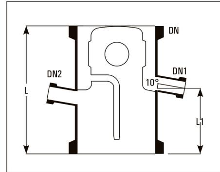
DN2 is used for insertion of a thermometer pocket. A bellow is recommended on the distillate outlet DN1.
