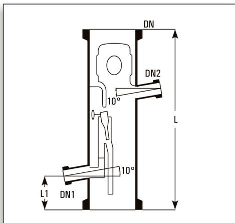
These reflux dividers are to be used with an electro-magnet and a timer. These have a swinging funnel mechanism which is operated magnetically from outside to remove the condensate or to return the reflux. Through this, correct control of reflux-ratio is possible. Funnel remains at 100% reflux position while magnet is inactive.
