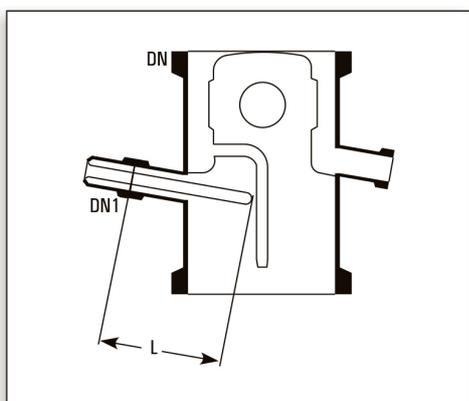
These thermometer pockets are to be used with reflux dividers or column sections. DN refers to the nominal diameter of the Reflux divider or Column.
